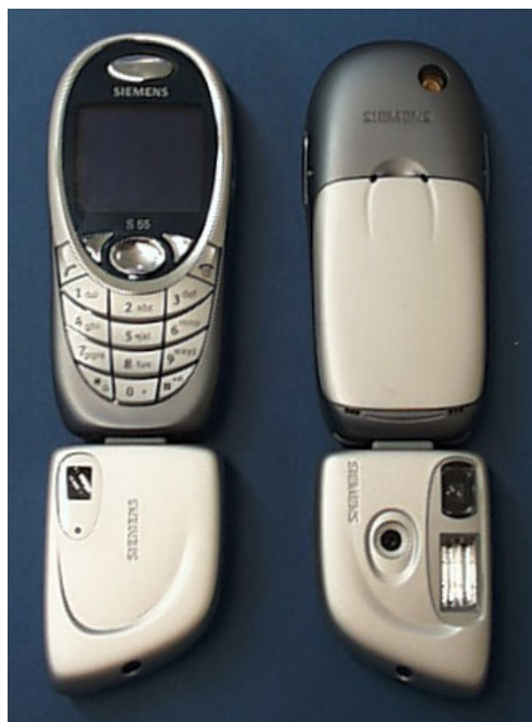
Fig. 26: Front and back view of the device with QuickPic Camera.
