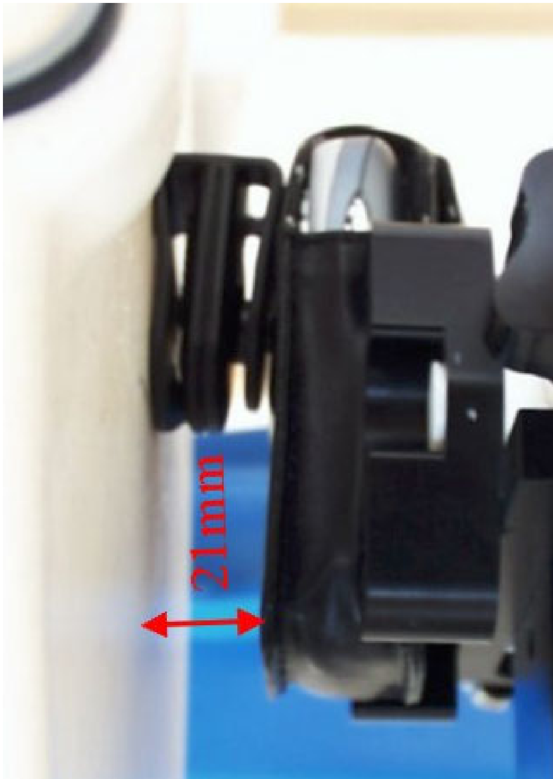
Fig. 47: Body worn configuration, Leather Case without Headset, (1 TX slot / 2 TX slots), Display up.
