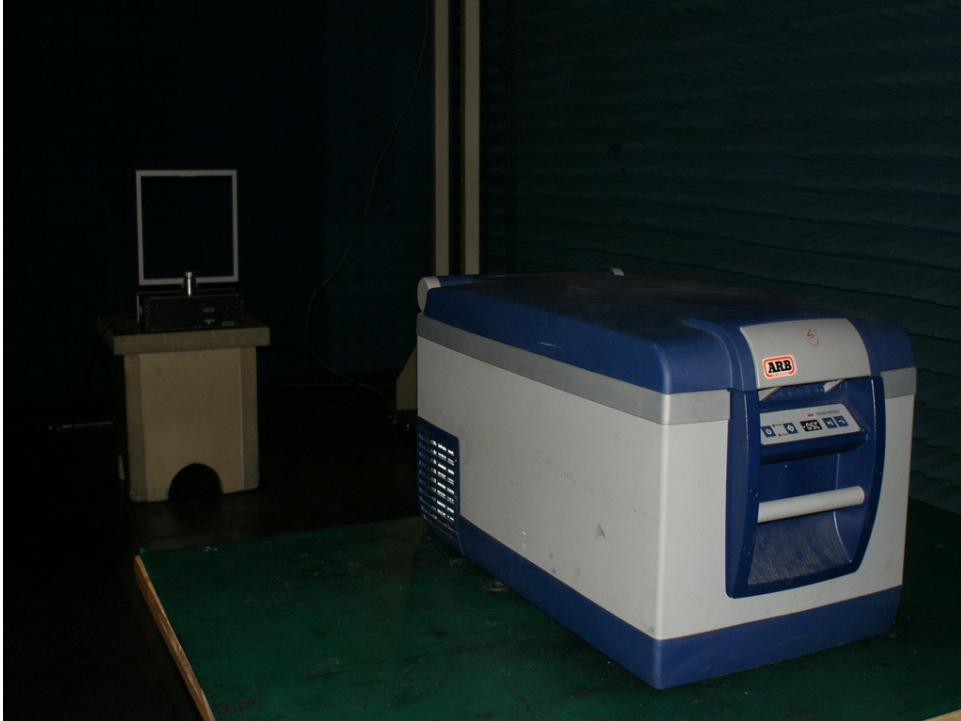
Photograph 2: Set-up for Spurious Emissions (30MHz-1GHz)
