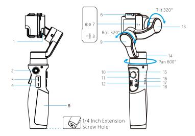
1 Mini LISB DC out Port 7 WiFi Indicator 13. Tilt Motor 8. WiFi Control ON/OFF 2 1/4 Inch Extension Screw Hole 14 Pan Motor 3. Trigger Button 9. Roll Motor 15. Bluetooth Liaht 4. USB DC Out/ DC In 16. Power Indicator Light 10. Mode Light 5. Handle (Battery inside) 17 Mode Button 11. Joystick 6 Thumb Screw 12 Slider 18. ON/OFF (Shutter button)
