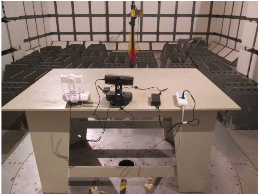
Radiated Emissions – Rear View (Above 1 GHz)
