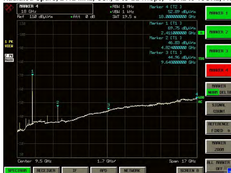
Radiated Spurs, 2412 MHz, CCK, 1 to 11 Mbps, 1GHz to 18GHz, Average plot
