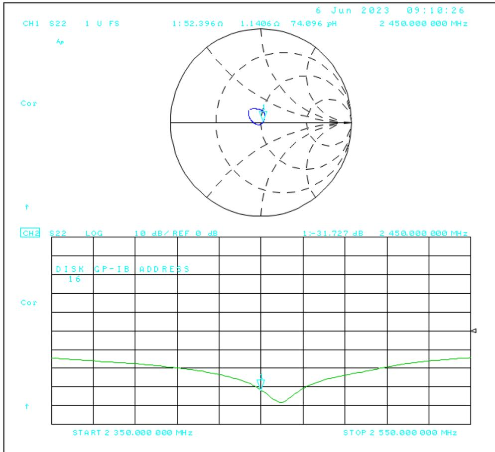
**5 Calibration report “5GHz System check dipole”**
