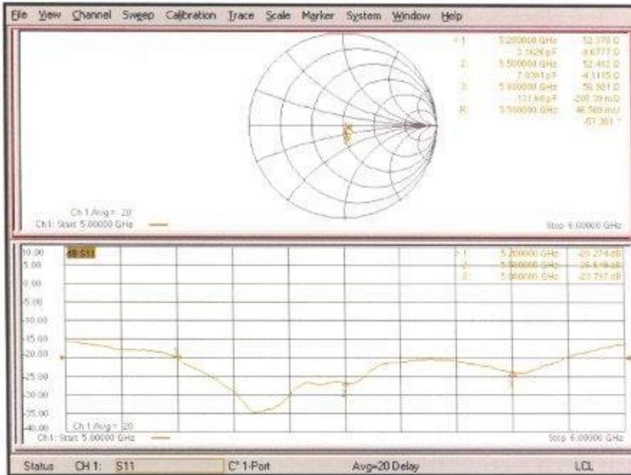
**Antenna Parameters with Head TSL at 5200 MHz**
