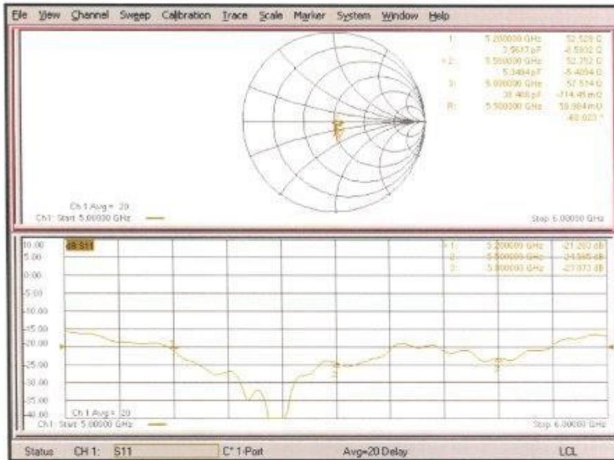
**Antenna Parameters with Body TSL at 5200 MHz**
