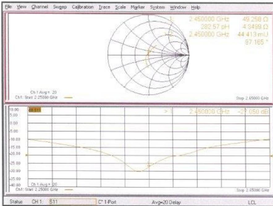
Antenna Parameters with Head TSL
