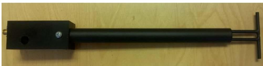
Figure 1 – MVG COMOSAR Validation Dipole
