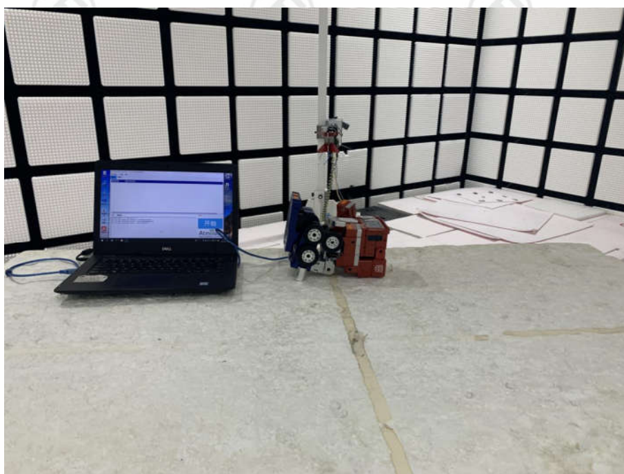
Radiated spurious emission Test Setup-2(Above 1GHz)
