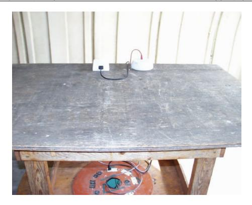
Radiated Emission below 1 GHz Measurement with Power Supply Model 6012
