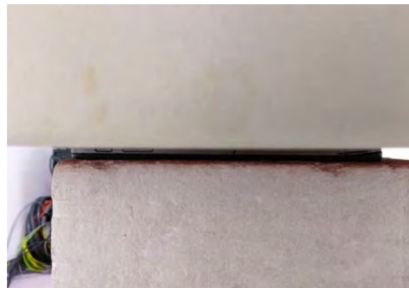
Fig.4 EUT Back side to flat phantom
