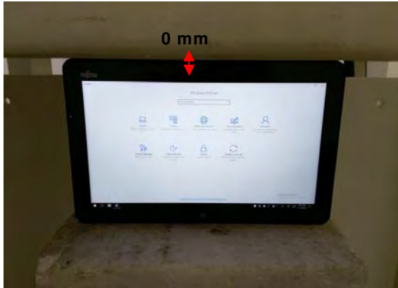
Fig.3 EUT Top side to flat phantom
