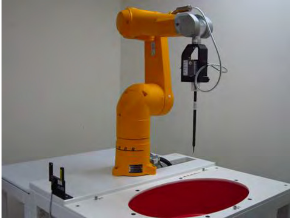
Fig.1 Photograph of the SAR measurement system
