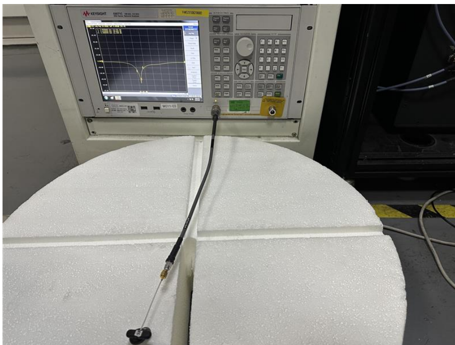
Free Space Right Impedance Setup
