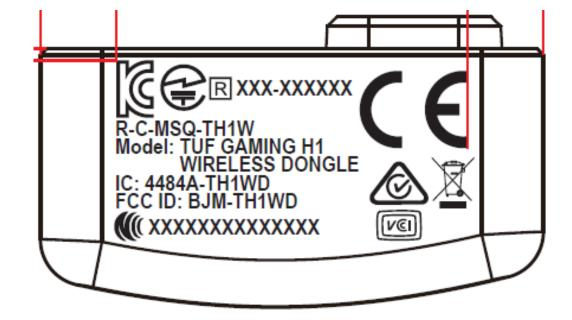
The FCC ID will be placed on the equipment as shown in the photograph below.
