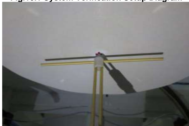
Fig.10.2 Photo of Dipole setup
