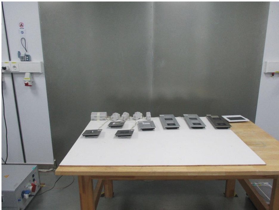
Setup photo of conducted emission (150KHz-30MHz)
