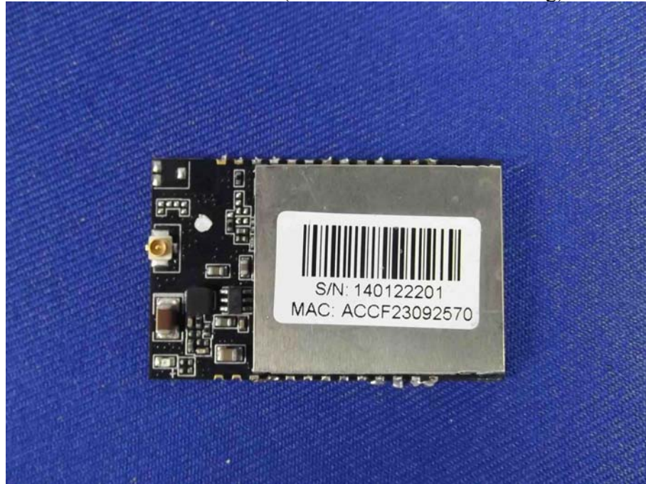
Figure 12 PCB of The EUT-Front View (WiFi Module With Shielding)
