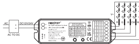
Controller connect to RGB+CCT LED strip diagram
