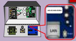
Tip: The intercom ID number can be found on a sticker beside the LAN port connection. (RJ45 connector may need removed to see the full ID.)
