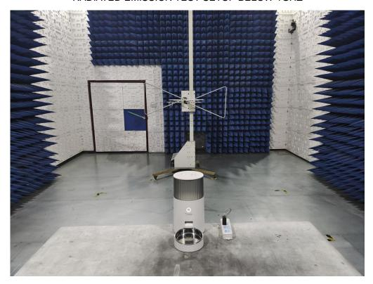
RADIATED EMISSION TEST SETUP ABOVE 1GHZ
