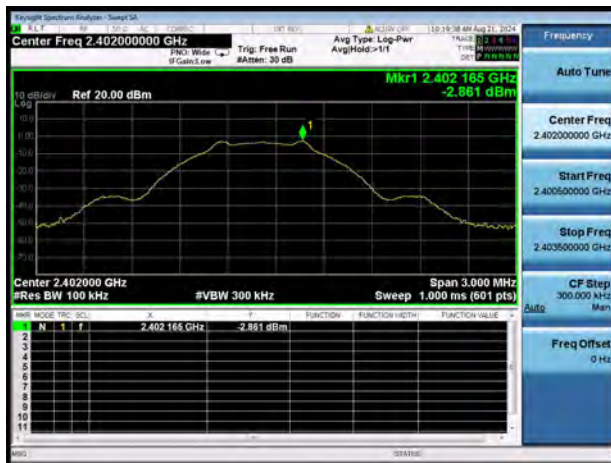
GFSK LOW CHANNEL, CARRIER LEVEL
