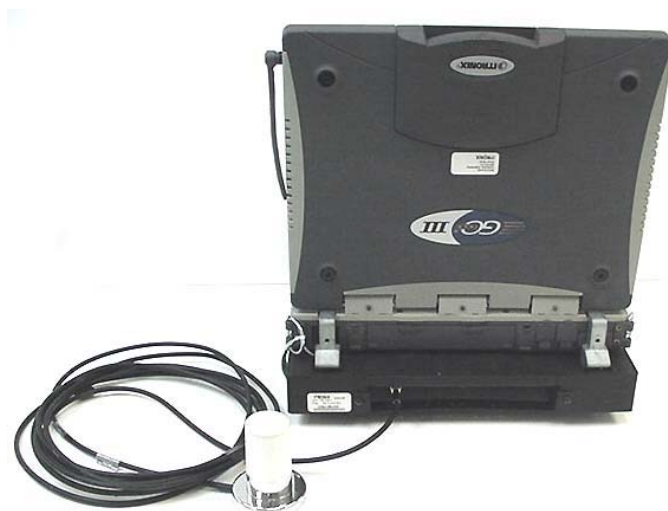
Photograph A.1-4 - DUT in Vehicle Cradle with Vehicle-Mount Antenna - back
