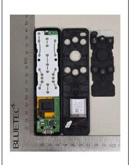
The difference is simply the number of CP (Content Provider) buttons on the exterior of the case. The internal circuitry is exactly the same.
