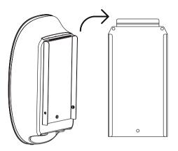
4) Lock the 2 x M4\*12mm screws on two sides.
