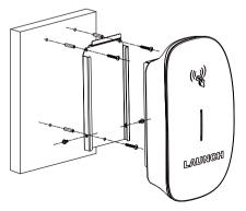
3) Insert the upper edge of the mounting bracket into the rectangular opening on the back of the charger to hang the charger.
