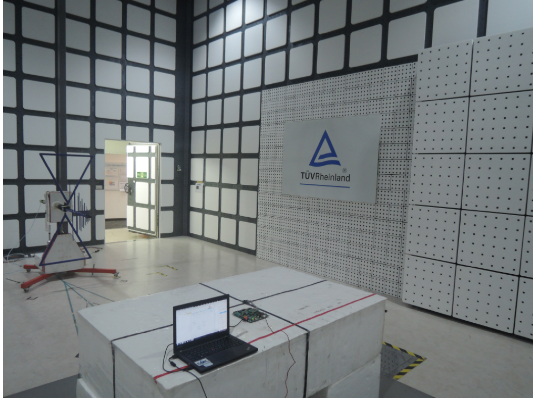
Set-up for Spurious Emissions (Back View 2) – without shield
