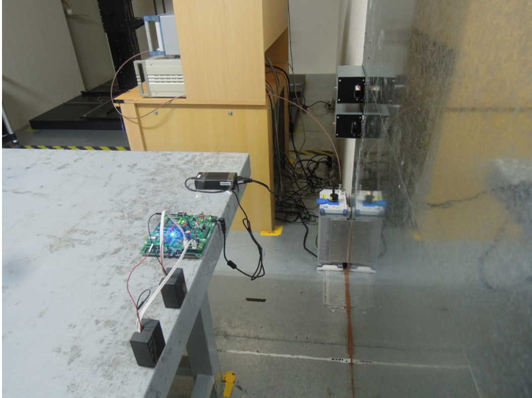
Set-up for Mains Conducted testing (Front View)
