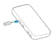
2. Pull out the card tray and place the nano-SIM card on the tray, as shown. Carefullyslide the tray back into place.
