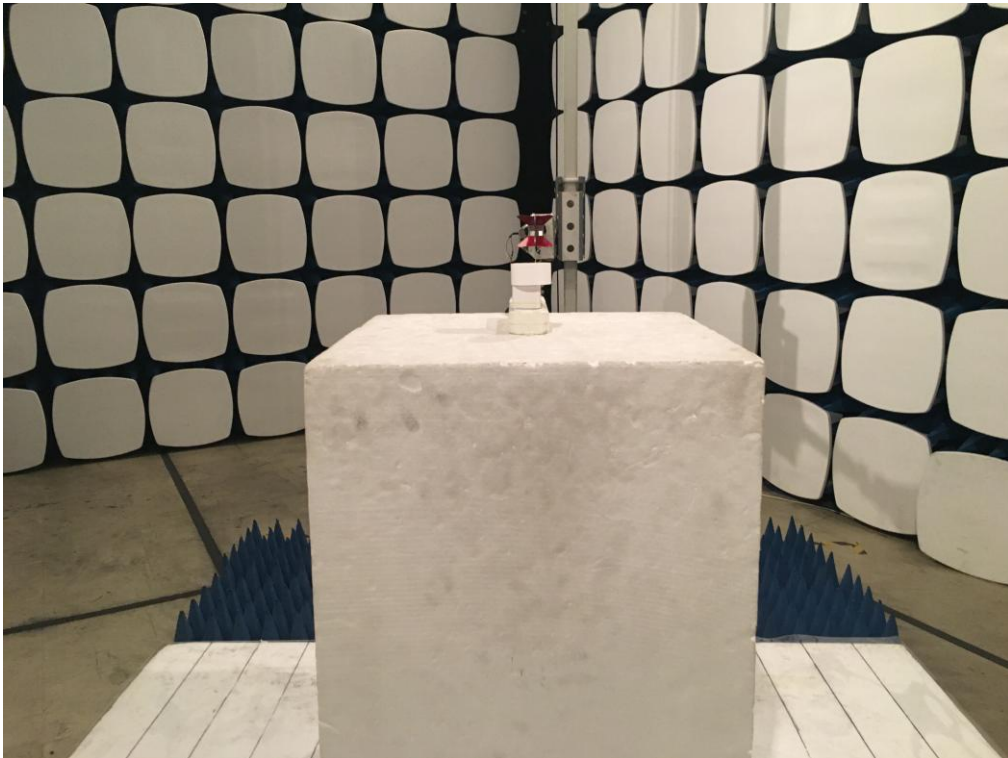
FCC RADIATED EMISSION TEST SETUP ABOVE 1GHZ
