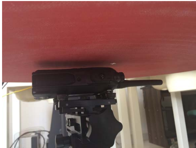
Face-held, The EUT display towards phantom 25mm
