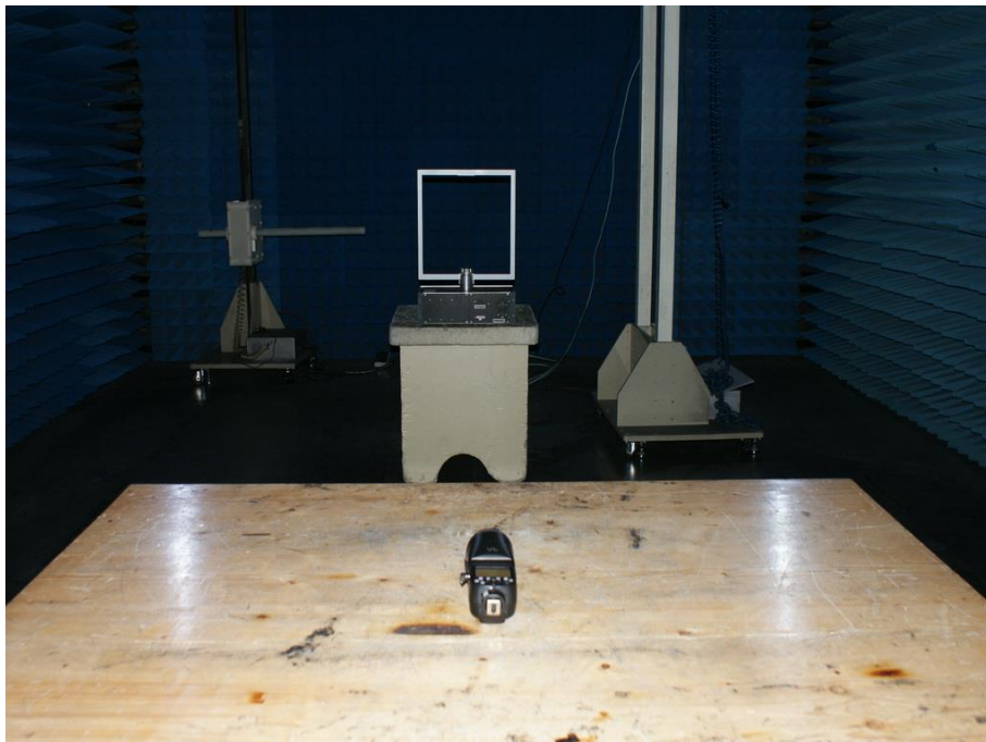
Photograph 2: Set-up for Radiated Spurious Emission, 9KHz - 30MHz
