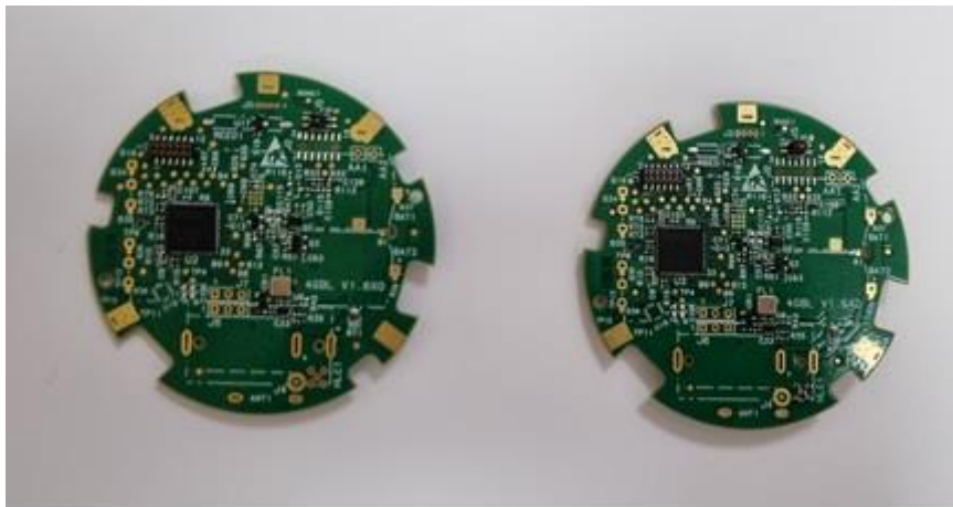
RF card-top, identical for both antenna configurations
