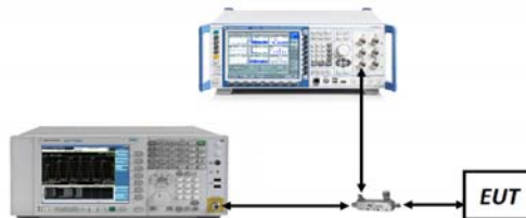
Figure 7-2. Test Instrument & Measurement Setup
