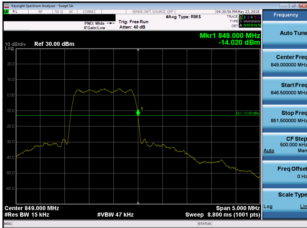
Plot 7-80. Band Edge Plot (Cellular CDMA Mode - High Channel)
