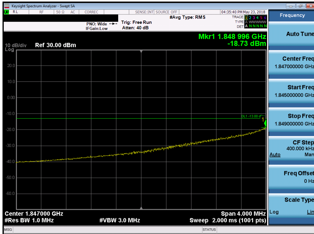
Plot 7-82. 4MHz Span Plot (PCS CDMA Mode - Low Channel)
