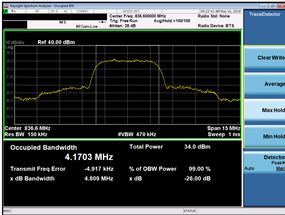
Plot 7-7. Occupied Bandwidth Plot (Cellular WCDMA Mode)
