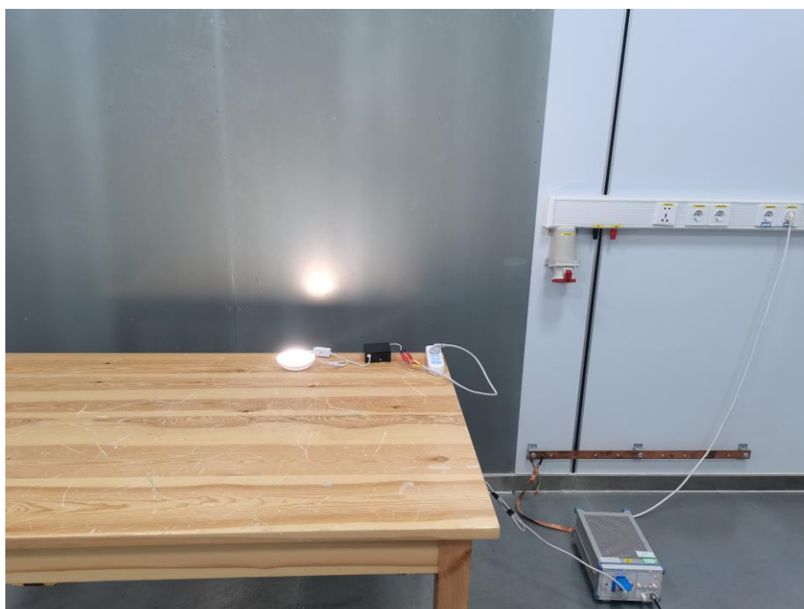
Fig. 4 Power line conducted emission setup photo
