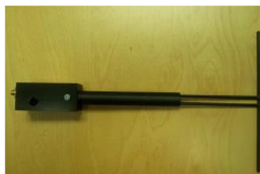
Figure 1 – MVG COMOSAR Validation Dipole
