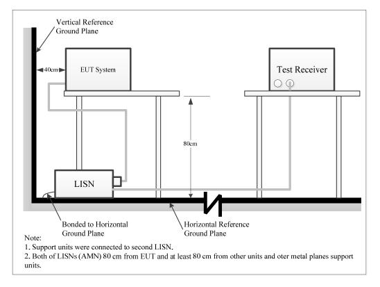
The setup of EUT is according with per ANSI C63.10-2013 measurement procedure. The specification used was with the FCC Part 15.207 limits.
