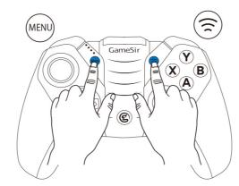
Clear Pairing: Before connecting the controller to other devices, please clear the previous paired device by holding down the Pair Button + MENU at the same time for 5s. Connect to New Devices: After clear the previous paring, follow the step of connecting devices for the first time.
