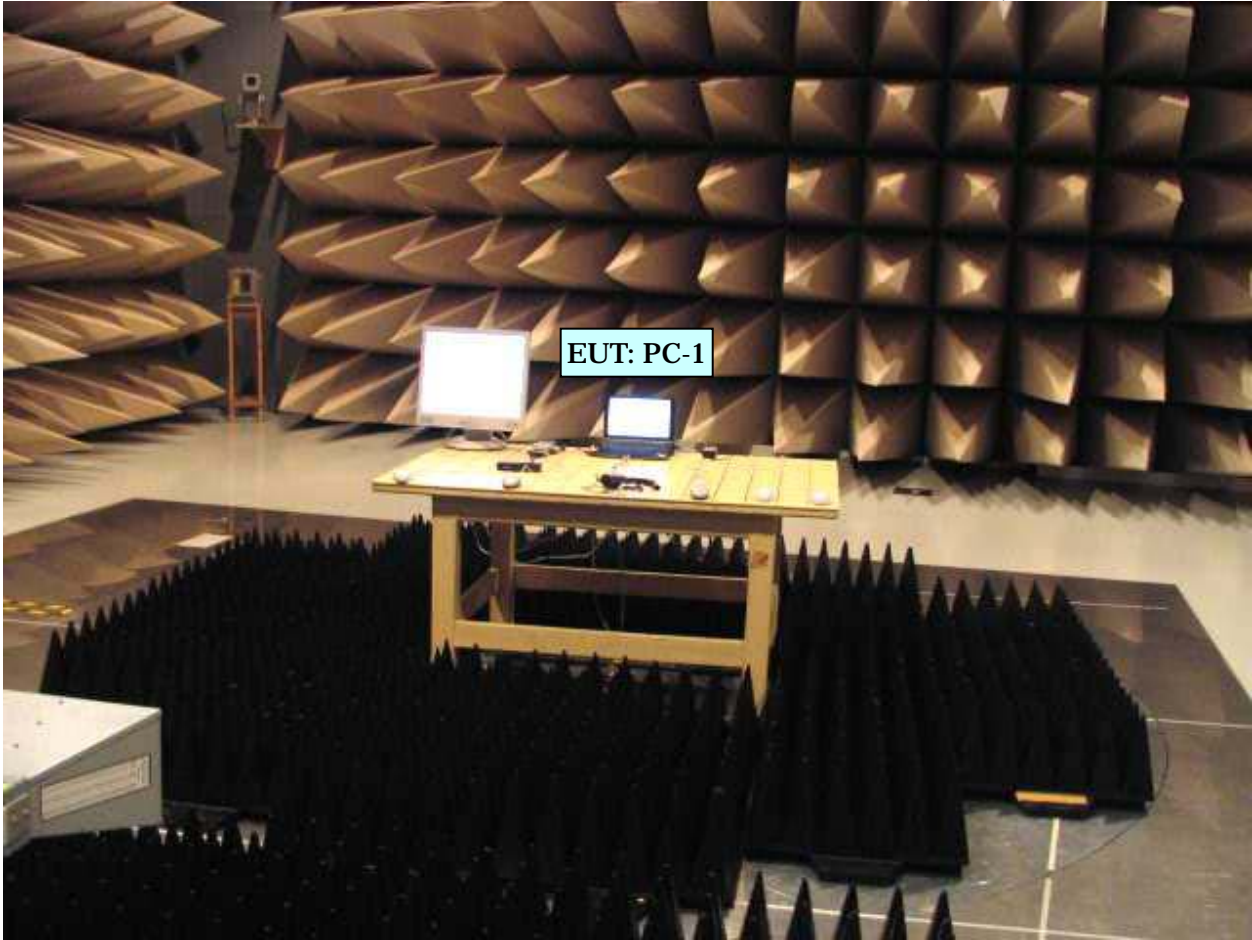
Photo-2.1 Conducted emission measurement
