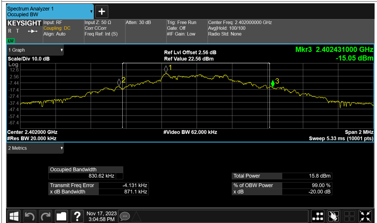
-20dB Bandwidth NVNT 2-DH1 2441MHz Ant1
