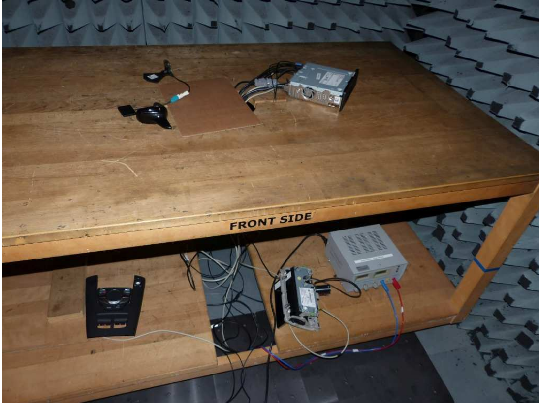
Photo 1: Test setup for radiated measurements (below 30 MHz)
