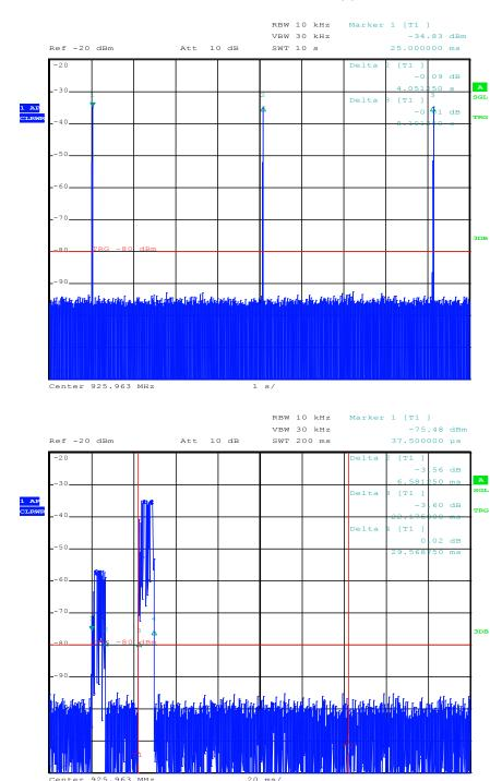
Note: The higher packets emitted from the EuT (the lower are emitted from the MWR wrench)
