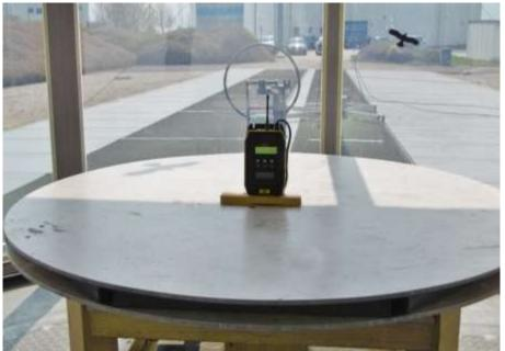
Test setup 30 MHz – 1000 MHz:
