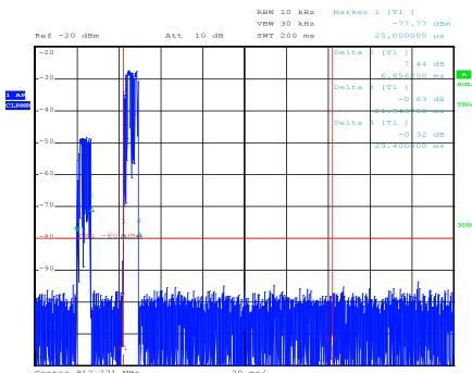
Note: The higher packets emitted from the EuT (the lower are emitted from the MWR wrench)
