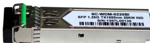
1000Base-BX WDM Singlemode (TX 1550 nm – RX 1310 nm)
