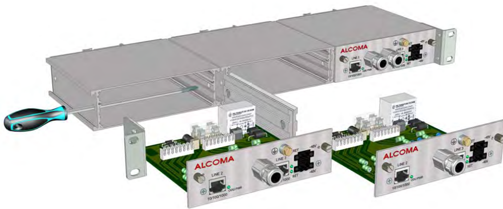
Figure 6 Assembling the three ALS1-GEth or ALS1-2GEth to 19" 1U unit
