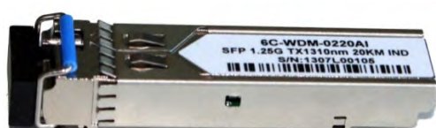
1000Base-BX WDM Singlemode (TX 1310 nm – RX 1550 nm)
