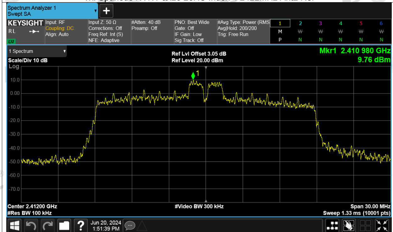
Tx. Spurious NVNT ax20 26RU Index 4 2412MHz Ant2 Emission
