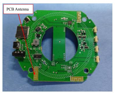
NOTE: The other two antennas receive microphone signals.
