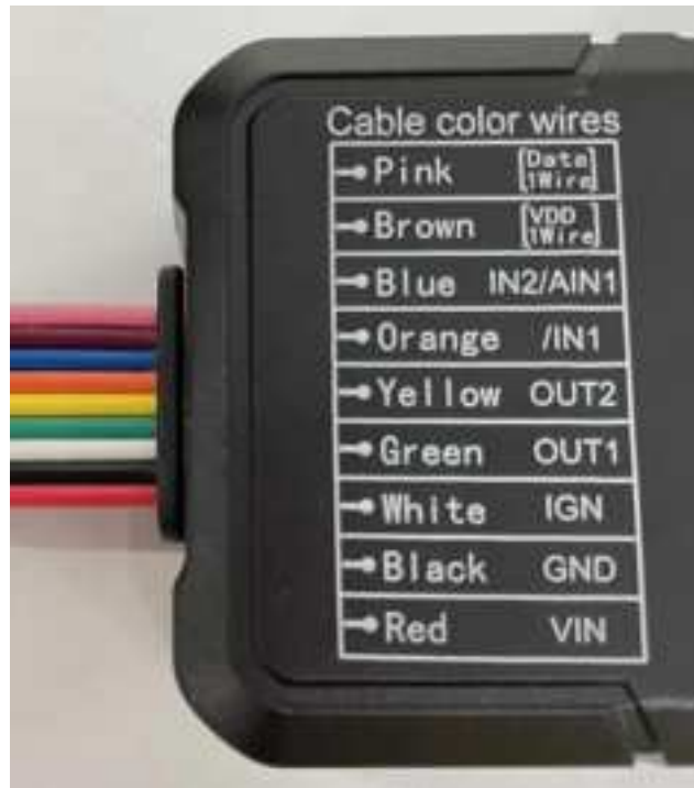
Figure 2: 9-PIN Wire Harness of GV58CEU
