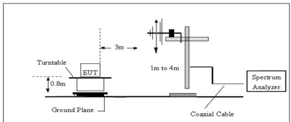
3. Radiated Emission Test-Up Frequency Above 1GHz
