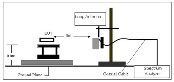
2. Radiated Emission Test-Up Frequency 30MHz~1GHz
