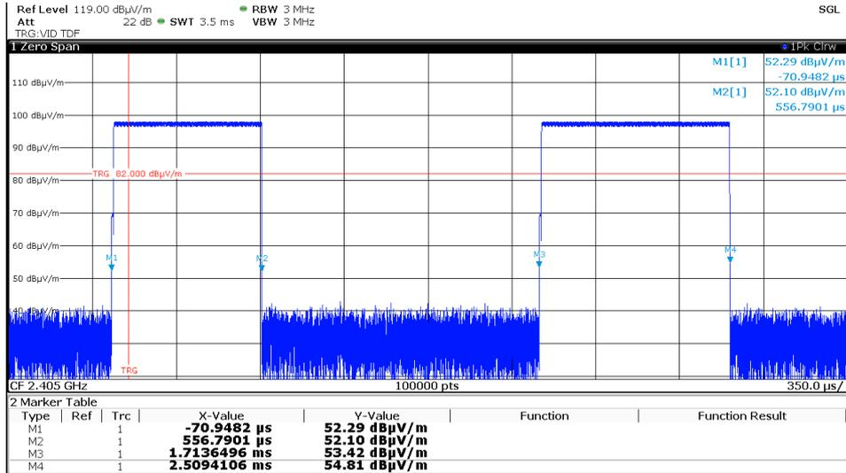
2 separate single pulses in a 100ms observation interval:
