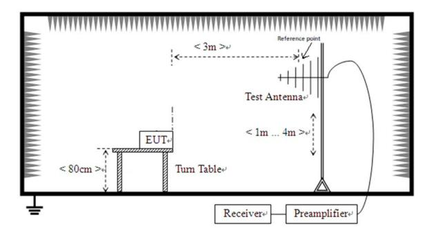
(For Radiated Emission Test (30 MHz-1 GHz))
