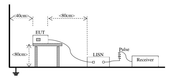
(For Conducted Emission, AC Ports Test)
