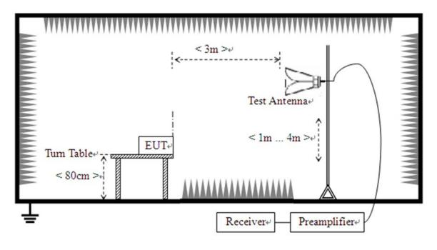
(For Radiated Emission Test (above 1 GHz))
