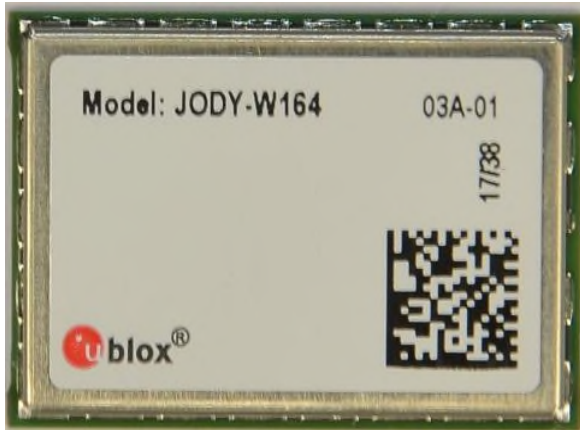
Figure 3: JODY-W164-03A top view external photo
