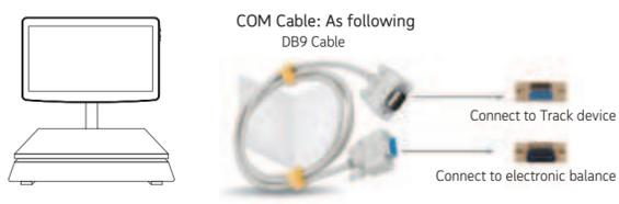
Can be connected to the Tracker and the Electronic balance by the COM cable, and then the Electronic balance will transfer the weight data to Tracker. At this time, the Tracker will calculate through the corresponding app application software, and display in the corresponding form in the Tracker.
