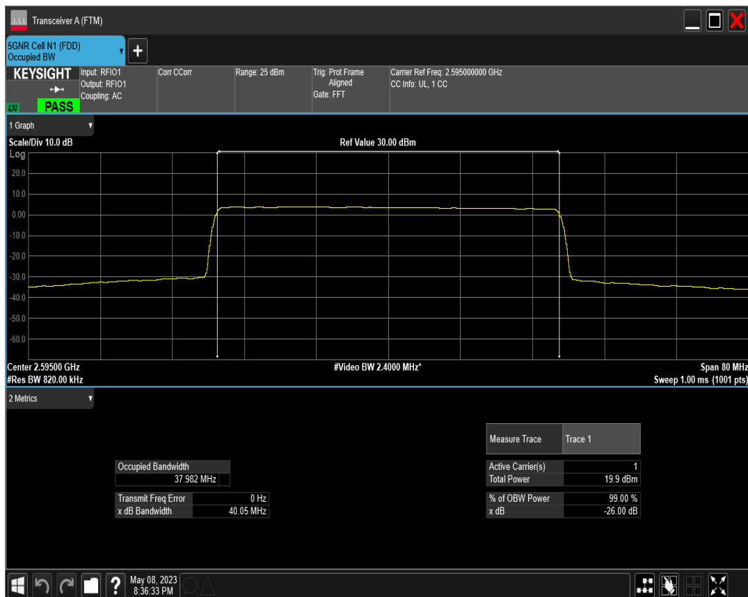
n38 SCS=30kHz DFT_BPSK BW=40MHz Channel=520000 RB=100@0
