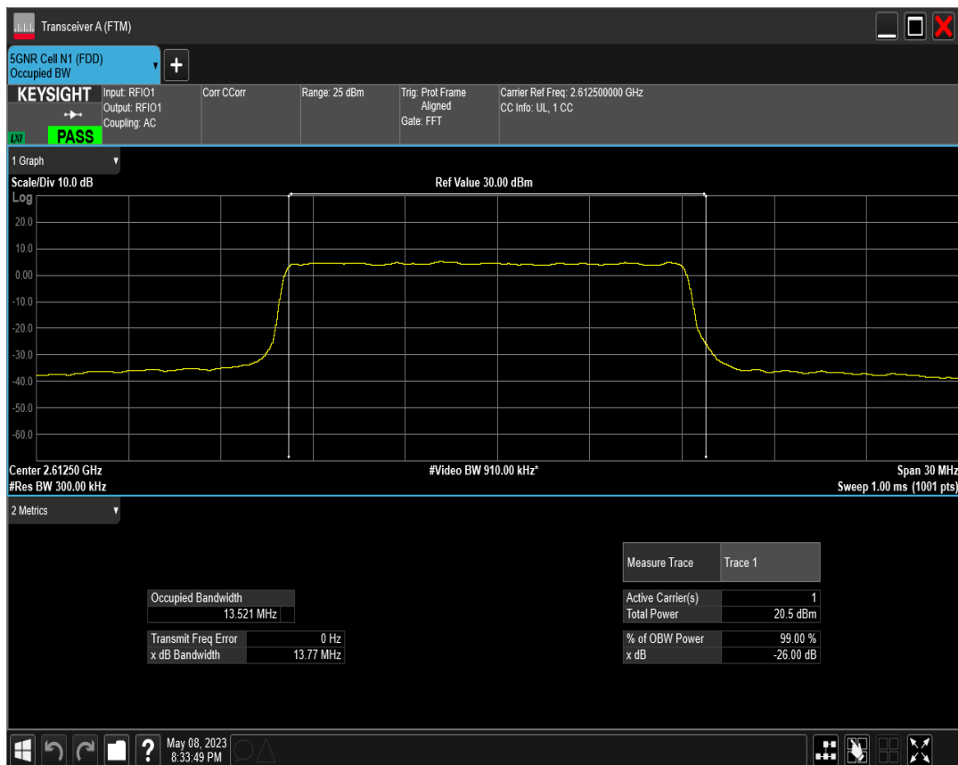
n38 SCS=30kHz DFT_QAM256 BW=15MHz Channel=522500 RB=36@0
