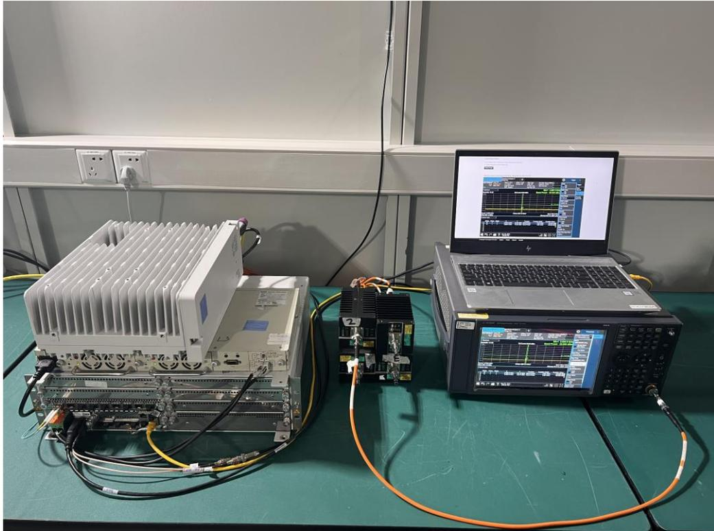
Description: Radiated Spurious Emission Test Setup for 9kHz to 30MHz
