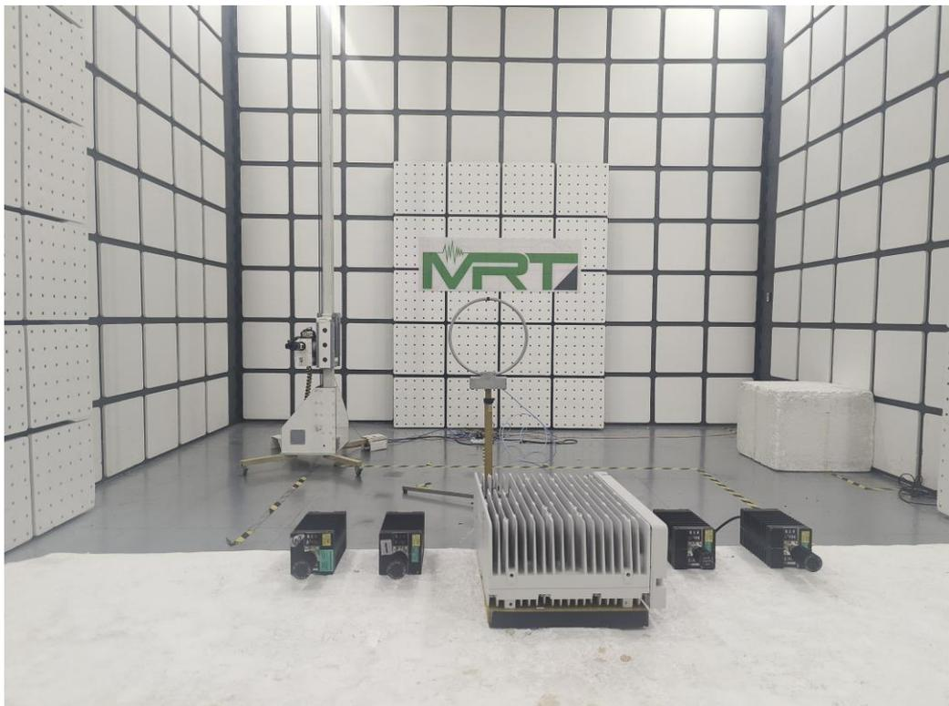
Description: Radiated Spurious Emission Test Setup for 30MHz to 1GHz
