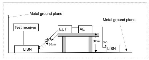
LISN: Line Impedance Stabilization Network
