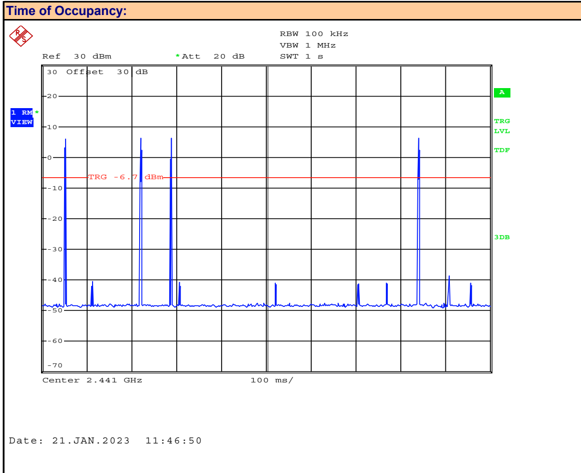
Plot 14.6 – Time of Occupancy, DH5, 2-DH5, 3-DH5, DM5
