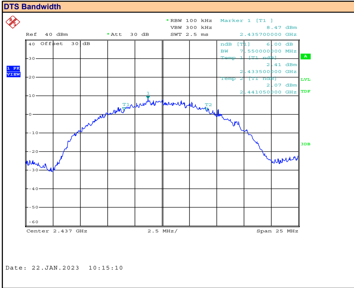
Plot 8.1 – 6dB DTS Bandwidth 802.11b
